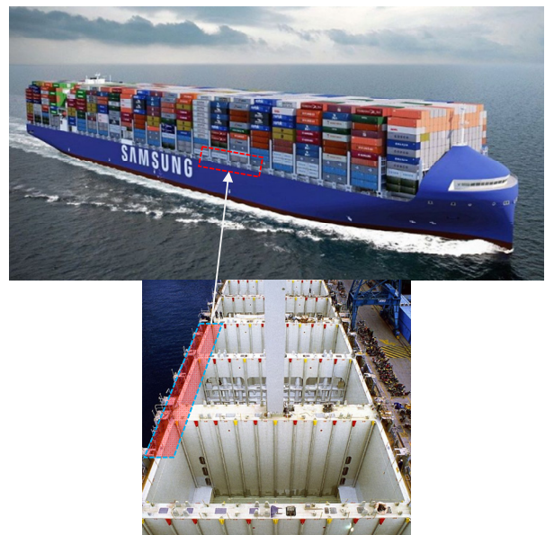
Fig. 1 Typical hatch coaming in the container ship
