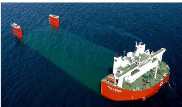
Fig. 2 HTV mobilized in load-out and float-off
